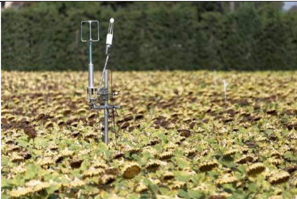
Figure 44: Flux tower on IINRA experimental sites
