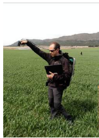
Figure 25: Taking radiometer measurement..
